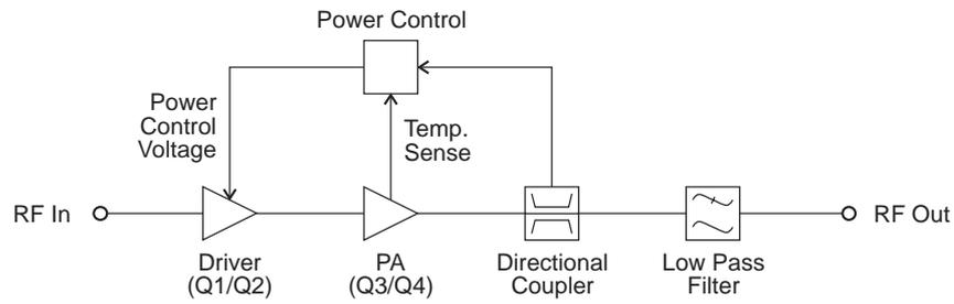
**Figure 2.1 T828 High Level Block Diagram**
